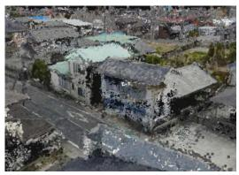
3D point cloud of a damaged house
