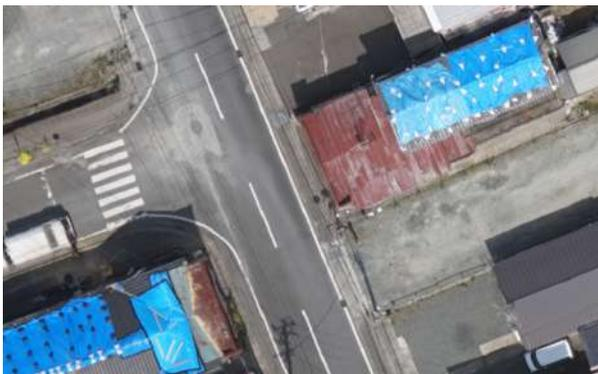
Orthomosaic showing damaged roofs are covered by blue sheet
