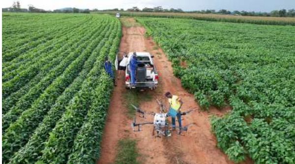
Refilling Drone spray tank with water and pesticide
