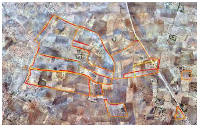
Surveyed farm boundaries on top of an orthomosaic
