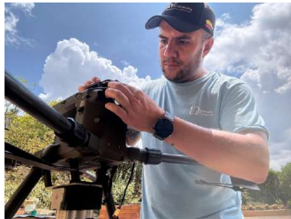
Altum multispectral camera assembly
