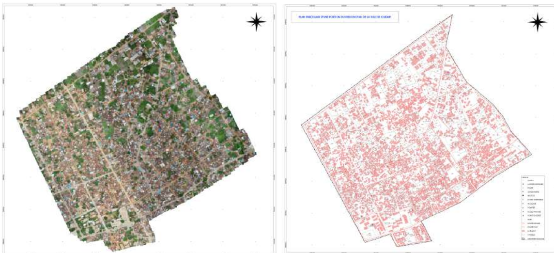
Data products created from drone data: orthomosaic (left) and plan of the area (right)
